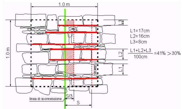
**Figure 7.2.8 Example of evaluation of effectiveness of connections between perpendicular walls (Source Angeletti, Borri, Longhi, Nasini, Severi (2004) "The law for seismic prevention in Umbria, Italy")**
