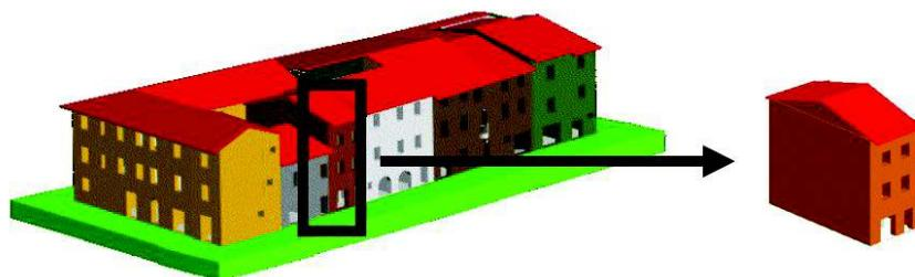
**Figure 7.2.5** The aggregation could be defined as a construction delimited by open spaces (left image). It is formed by Structural Units (U.S.) which could be defined as portions of the aggregation which have a Unitarian static and seismic behaviour.
