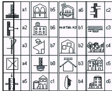
**Figure 7.2.12 Symbols representing the structural deficiencies of the aggregation**
