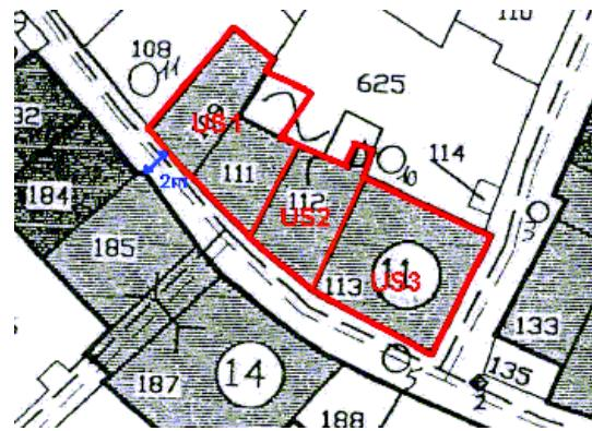
**Figure 7.2.13** In this figure it is possible to see a panoramic view of the aggregation. Its dimensions are approximately 30m x 11m. It is formed by three U.S. Each U.S. is a four storey masonry building.
