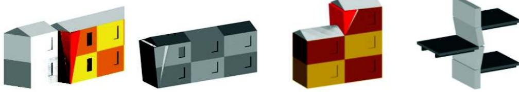
The not aligned facade causes a wall not to be buttressed by the other buildings.
